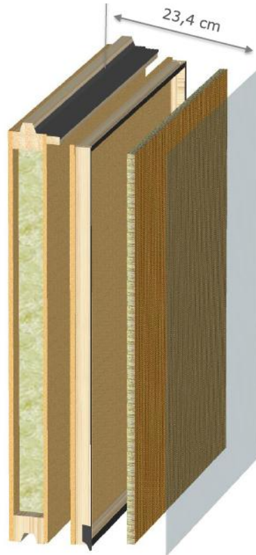
Figure 3.1.3: GAP:skin for renovation projects (GAP 3 Solutions 2016).
