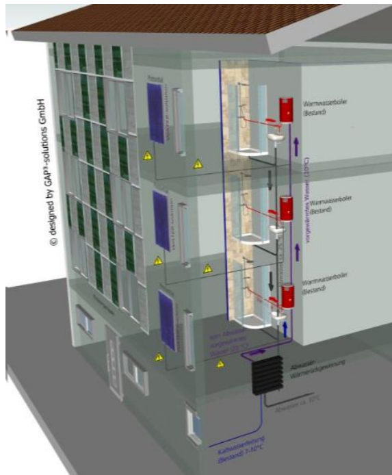
Figure 3.1.6: GAP:water PV, overall connection with Waste Water Energy Recovery System (GAP 3 Solutions 2016).
