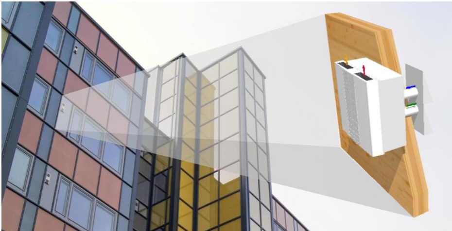
Figure 3.1.4: GAP:air element, where the white box is placed on the inside of the wall (GAP 3 Solutions 2016).
